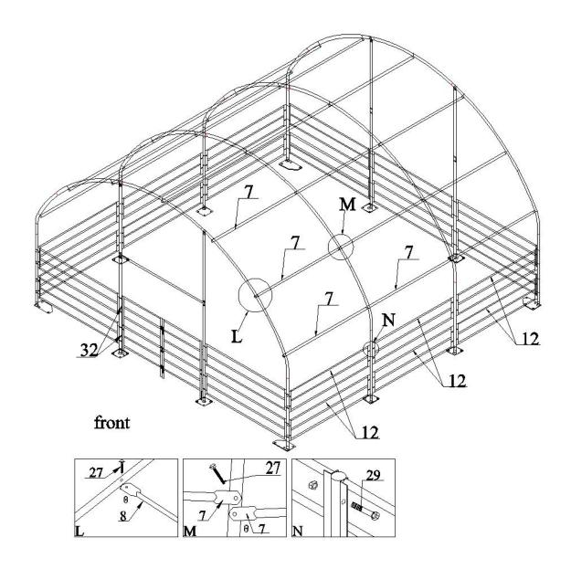
Step 6: squaring up the frame and fix base plates by stake peg
