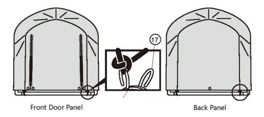
7 Tie the other side of the roof cover rope end on parts #16 also (drawing A), and then through the door panel eyelet and tight again(drawing B).
