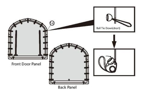
Following below diagram to attach the roof cover. Please pay attention to the cover direction, the eyelets are on the two sides of the shed.
