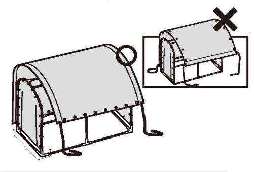
Tie one side of the roof cover rope ends on parts #17.
