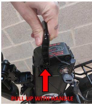
Remove battery by pulling up using the battery handle. (You will need to lift the saddle into the upright position to remove the battery. Lift the blue lever under the back of the saddle to do this.
