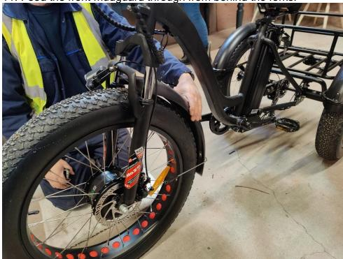
12. Unscrew the bolt that holds the front light in place and re-attach with the mudguard in place.
