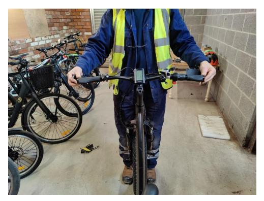
Straddle the front wheel (as seen in picture) by standing in front of the trike. This prevents the front wheel from moving when making adjustments to the handlebars. Align the handlebars so they are straight with the front wheel. Tighten as necessary.
