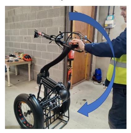
6. Align the front wheel to fit in the grooves of the forks. This will slot into place. Be sure to check that the wheel is the correct direction (refer to the arrow on top of the wheel hub to see which direction is forwards.
