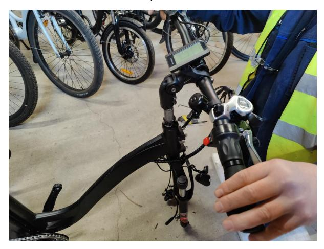
3. Use the provided tool to tighten the handlebars into the frame. Tighten loosely as adjustment to straighten the front wheel may be required.
