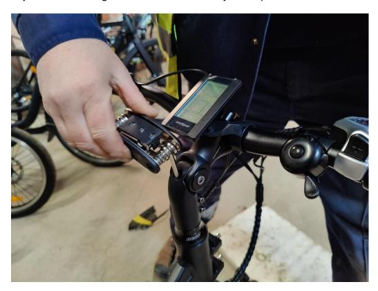
4. Tighten the two screws as seen in the picture to secure handlebars. Again, tighten loosely as further adjustment to straighten the front wheel may be required later.
