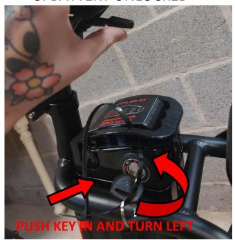
To unlock the battery, push the key in and simultaneously turn anticlockwise / left until it clicks.
