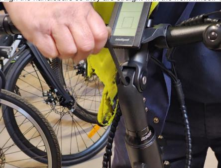
11. Feed the front mudguard through from behind the forks.
