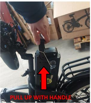
Remove battery by pulling up using the battery handle. (You will need to lift the saddle into the upright position to remove the battery.
