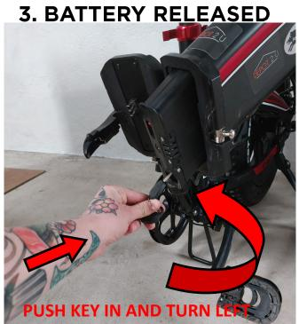
To remove the battery, push the key in and simultaneously turn anticlockwise / left until it clicks.
