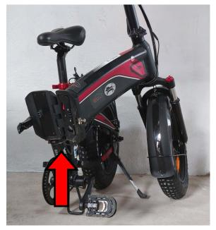
The battery is situated inside the bike frame To located—unclip the lock on the middle of the frame and fold the bike to expose the battery compartment
