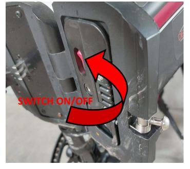
To turn battery on or off—Use the red switch located inside the battery panel
