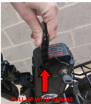
Remove battery by pulling up using the battery handle. (You will need to lift the saddle into the upright position to remove the battery.
