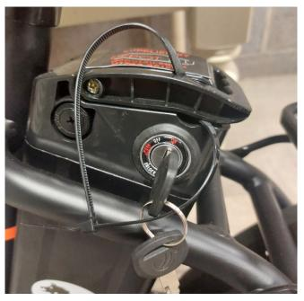
Key in 12 o'clock position means the battery is switched on. The battery must be switched on to turn the bike on, which is done on the control pad by pressing and holding the power button.
