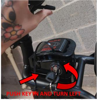
To unlock the battery, push the key in and simultaneously turn anticlockwise / left until it clicks.
