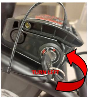
To turn battery off, turn the key anticlockwise / left until it clicks.
