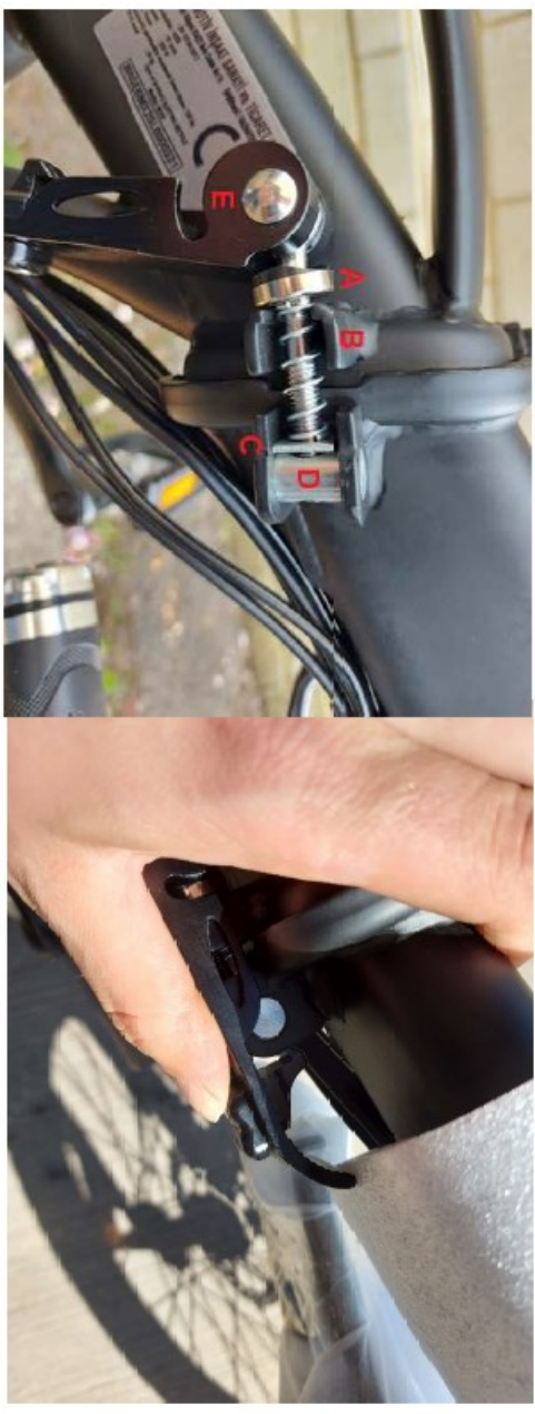
2. Lock center Bike hinge with clamp - this should be secure and not wobble. If adjustment is needed, turn the pin (E) clockwise / counterclockwise to tighten / loosen.
