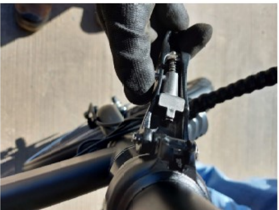
3. Lock handlebar stem in place with spring lock.
