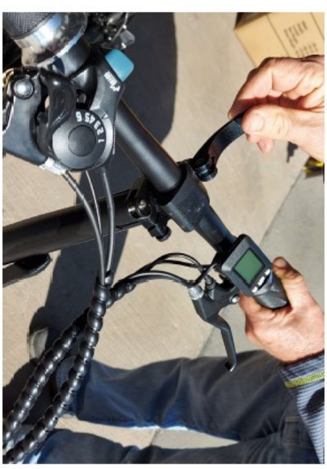
4. Adjust height and angle of handlebars by unlocking collar and turning appropriately
